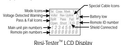
Instructions for Use Resi-Tester<sup>TM</sup> powers off automatically 9 minutes after the last button press in cable testing modes and after 2.4 hours in tone mode. Be sure to install a battery if using for the first time, see battery installation section.
