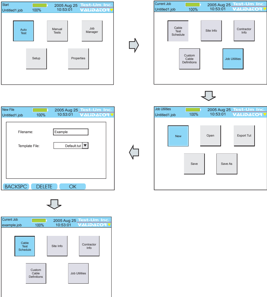
Figure 3.3 Creating a New Job Flowchart
