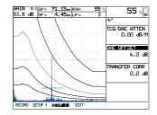
Tools for easy defect sizing Multiple curve DAC shows recorded DAC curve in magenta with 4 additional curves based upon dB Offset feature for added flaw sizing assistance. TCG Attenuation and Transfer Correction features make it very versatile for use on other materials and surface conditions.
