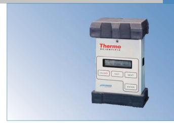
The Thermo Scientific personal DataRAM pDR-1000AN Monitor is a passive sampling, light-scattering nephelometer that measures real-time mass concentrations of dust, smoke, mists, and fumes in industrial as well as other indoor and outdoor environments.
