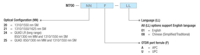
Specify power cord type (country) when ordering an M700 OTDR. One power cord is included with each AC adapter at no charge.
