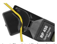
Insert fiber into LFI channel and pull trigger on unit to initiate macro bend in fiber. The LFI does not cause excess loss in the network.
