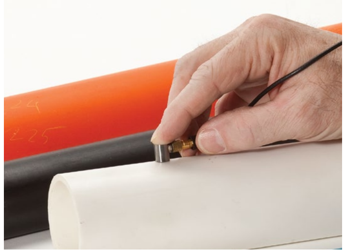
Measure the thickness of many materials including plastic, metal, rubber, glass, ceramic, and composites.
