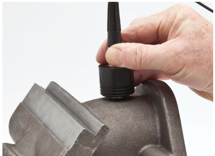
Many cast metal parts or sound-attenuating materials can be measured with the High Penetration software option.
