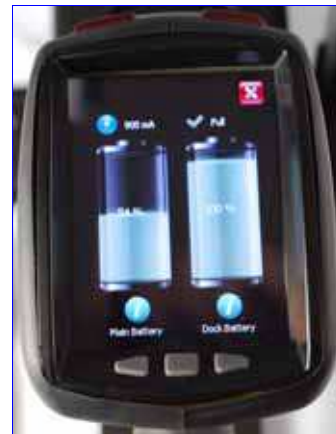
Battery Status Screen (Delta inserted in DDS)
