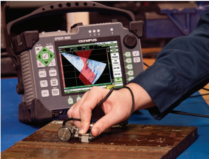
Phased Array S-scan with Weld Overlay
