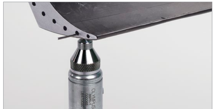
Measurement of a turbine blade using the wire targets
