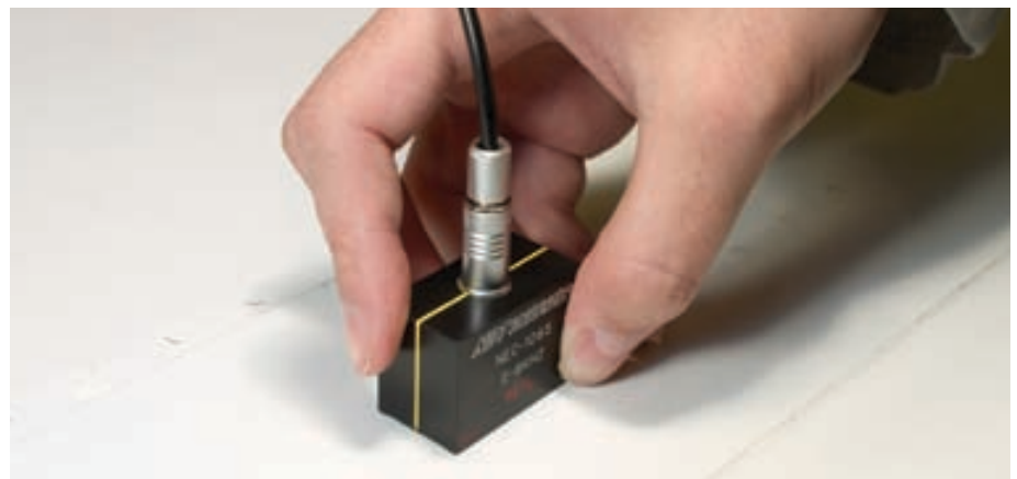
Surface preparation is minimal. Unlike liquid penetrant or magnetic particle inspection, it is unnecessary to remove the paint from the surface to inspect the parts.
