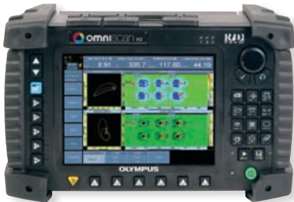
Fastener inspection using two frequencies and dual C-scan display.
