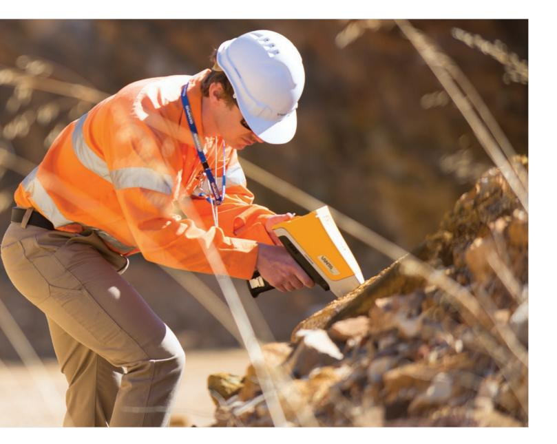
Olympus' new Vanta<sup>™</sup> analyzer is our most advanced handheld X-ray fluorescence (XRF) device. These rugged, powerful, and intuitive instruments provide rapid, accurate element analysis and alloy identifications to customers who demand laboratory-quality results in the field.
