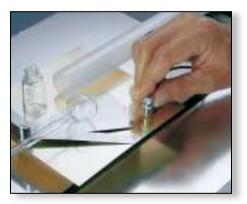
**Thin Material/High Resolution** The 25DL measures thin steel down to 0.006" (0.15mm) or plastic as thin as 0.003" (0.08mm).
