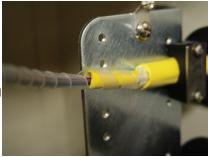
Macrobends, microbends, and breaks in an optical fiber will all radiate light to varying degrees depending upon strength of the tracer source, distance to the fault, and buffer characteristics. Dark fiber buffers may attenuate light escaping from a fiber discontinuity by several more decibels than a light colored buffer. The PX-B603 has variable gain to accommodate all common buffer styles.
