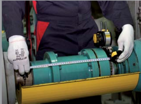
Enter dimensions The necessary sensor and machine foot dimensions are quickly inputted.
