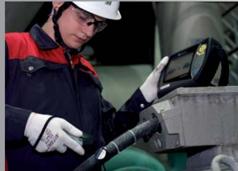
Save Updated machine data and alignment status are recorded on the RFID tag.
