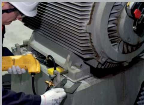
Vertical and horizontal alignment correction Simultaneous live monitoring of machine corrections in vertical and horizontal directions. PERMABLOC® shims in appropriate sizes simplify the process of raising or lowering the machine.
