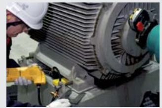
Optional: shims (left) and a lifter unit to lift machine to insert or remove shims.
