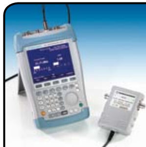
R&S®FSH with R&S®FSH-Z44 directional power sensor
