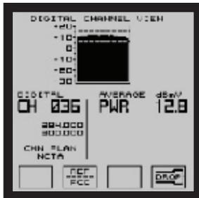
Quickly tune and display the average power of a single digital channel. The spectrum analyzer display shows how the power is distributed over the channel's bandwidth.
