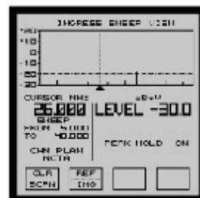
Check for ingress on the return-path. The spectrum analyzer display reveals the ingress signals that interfere with digital services such as VoIP and high-speed data.
