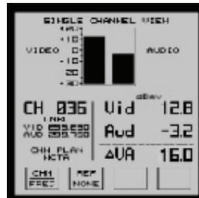
Quickly tune and display the picture carrier, audio carrier and dB difference on a single screen. Monitor audio quality on the built-in speaker.
