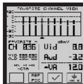
View only 'Favorite' channels for a quick snap-shot of the system. Press the 'check' key for an on-screen pass/fail summary.
