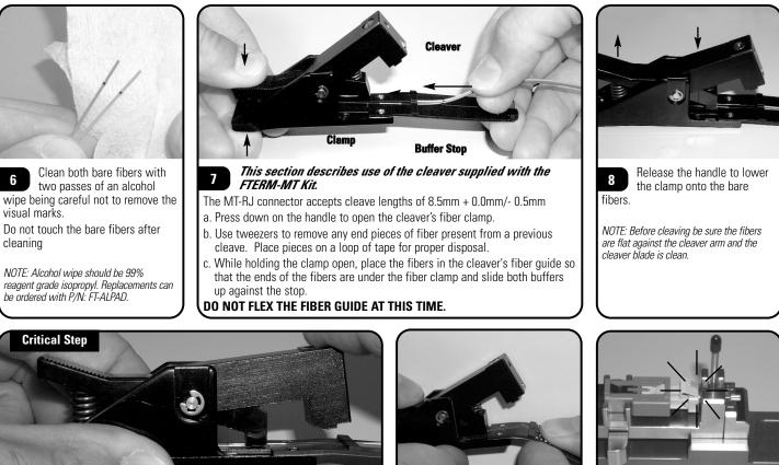
Gently press down the cleaver arm until it just touches the fibers and 9 guide then release. This will apply enough pressure to properly score the fibers. It is important that both fibers are scored equally. Excessive pressure on the cleaver arm during this process will improperly score the fiber and result in a poor cleave and high insertion loss during link testing. Do not put pressure on the clamp arm during the cleave.
