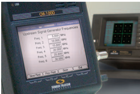
CM-USG Upstream Signal Generator Module
