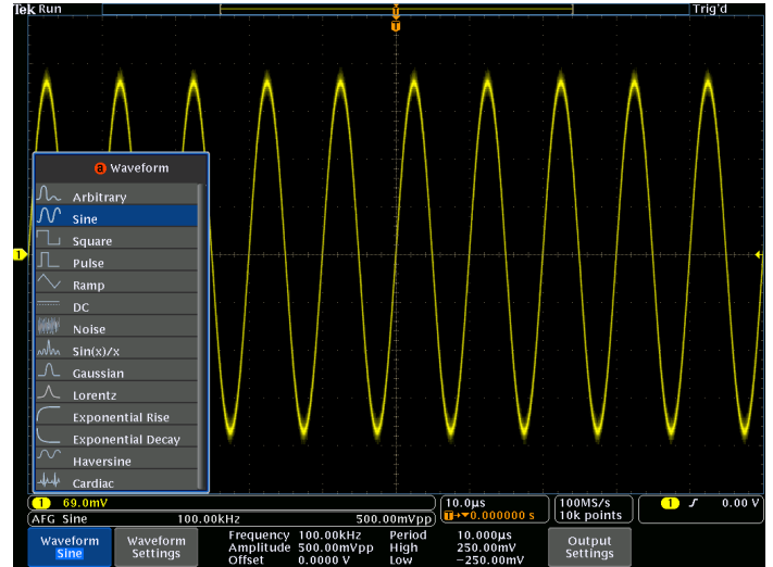
Waveform type selection in the integrated AFG.
