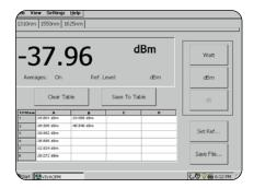
The YOPM, a PCMCIA-based Optical Power Meter, supports all your optical power measurement needs. It measures all common telecommunication wavelengths from 850 nm to 1625 nm. Easy saving of measurement data makes this an ideal tool for documenting networks.
