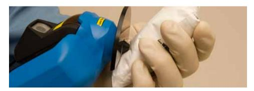
The TruScan analyzer's point-and-shoot operation enables sampling through packaging such as double-bagged pharmaceutical ingredients in a drum or tablets in blister packaging.
