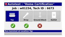
Multi-user support allows technicians that work in various territories to easily switch channel plans and standardized autotest apps and test limits or login as a completely different user. The built-in web browser allows techs to upload job data in near real-time as well as transmit and receive channel plans, autotests, work orders and firmware.
