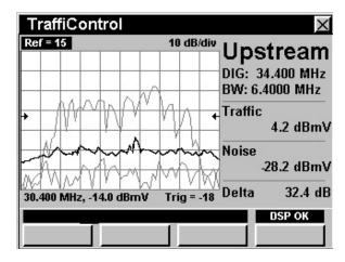
Find in-channel distortion or other interference without interrupting service with Error Vector Spectrum™ or TraffiControl™ modes.
