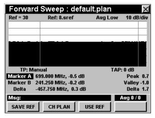
Measure system frequency response with SpeedSweep system compatibility.
