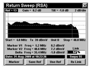
The 860 DSPi, with an SR-1 Option, injects an agile sweep signal configured to "step around" active channels, sweeping in unoccupied spectrum areas to a frequency resolution of 100 kHz. The reverse sweep is received by the 8310 RSA<sup>™</sup> and the response information is relayed back to the 860 DSPi on via user configurable frequency agile forward telemetry signal.
