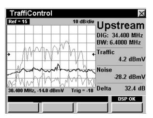
Find in-channel distortion or other interference without interrupting service with Error Vector Spectrum<sup>™</sup> or TraffiControl<sup>™</sup> modes.
