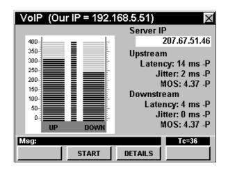
Measure latency, jitter, packet loss, and other VoIP parameters in seconds. Analyze VoIP performance from end-to-end and from the subscriber to the CMTS. When testing end-to-end, the 860 DSPi displays separate test results for upstream and downstream paths and even calculates an MOS score for each.
