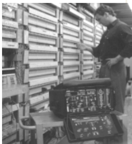
The T-BERD 310's extensive DS1 measurements enable you to qualify and troubleshoot digital circuits.
