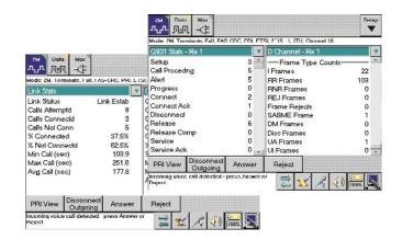
In both Emulate and Monitor modes, statistics are presented relating to channel utilization, number/percentage of calls connected, and other key parameters for satisfactory performance analysis.
