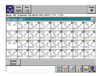
The 2M View provides a complete overview of the current state of the G.704 access, for example confirming activity (or the absence of), prior to taking the link out of service for essential services.
