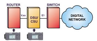
The 2230 replaces and emulates the customer's router or DSU/CSU to confirm satisfactory operation of the provided service.
