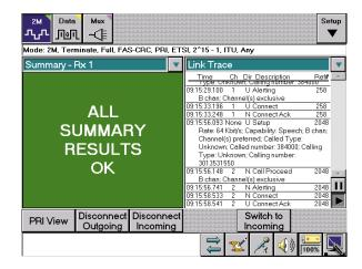
The Trace function captures relevant signaling information during emulation and monitor, to aid fault diagnosis by providing clear detail of the messages that led to a call failed.
