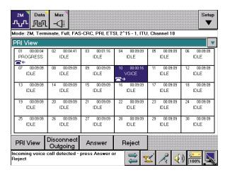
In View mode, the current status for all 30 channels can be seen at a glance. Activity is shown in real time.
