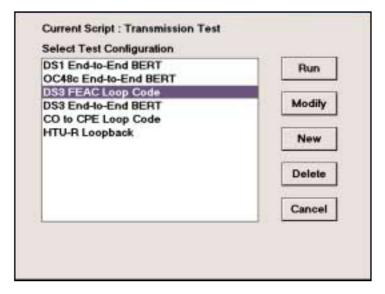
*Configurable Results* (*Quad Results*<sup>™</sup>)—Correlate results from multiple interfaces and payload mappings (SONET/DS3/DS1) and quickly assess network performance by using the 2310's configurable results features. It also provides functionality to analyze selected results simultaneously in up to four windows.
