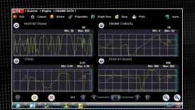
Touch any live data parameter to display in graph, text or full screen mode. View up to sixteen data parameters at once for true cause and effect diagnostics.
