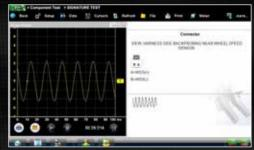
Exclusive Fast-Track Component Test Meter shows guided component test procedures, live scope readings and known good waveforms side-by-side.
