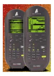
With the growing implementation of digital carrier transmission, guarding against ingress becomes more important. Most cable systems are implementing processes that require the installer to certify the installation by checking for leaks at the end of the install. This will insure that there are no leaks, and this correlates to no ingress. The CLI-950 can also be used by dedicated leakage crews, and with leakage GPS tracking systems.
