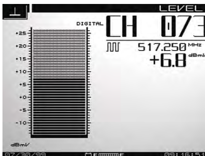
Digital channel average power measurements can be made using the digiCheck™ feature
