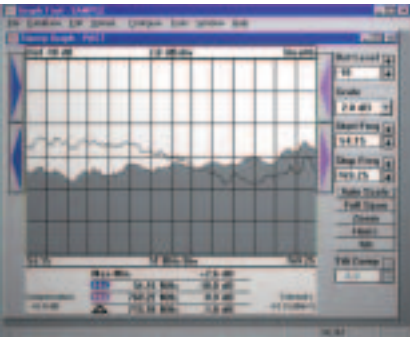
Detailed forward/ reverse sweep graph offers adjustable markers, scale, reference level and tilt. Users can clearly distinguish between previous and current sweep measurements for easy comparison on PC StealthWare display
