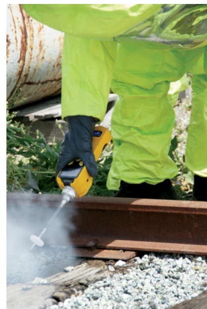
Workers can quickly measure VOCs and wirelessly transmit data via Bluetooth.
