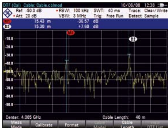
Distance-to-fault (DTF) measurement
