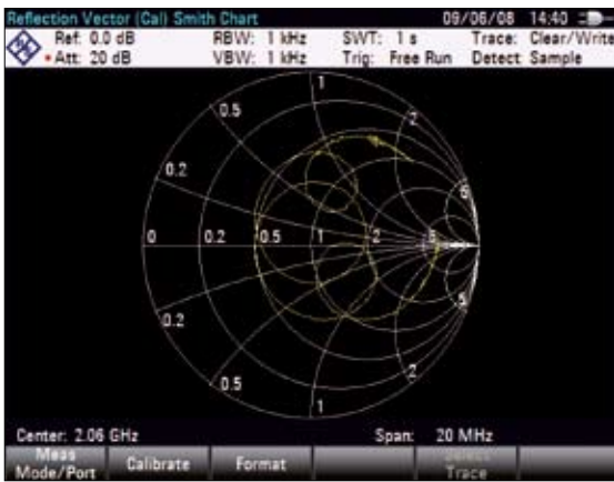
Vector network analysis: measurement with Smith chart
