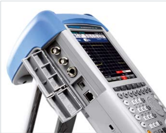
Additional connectors (e.g. for LAN and USB) are protected by caps
