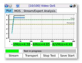
display of IP Video results. Tech-X Flex gives a Video MOS score (VMOS) which rates the customer's QoE with a number between 1 and 5. The closer to 5, the better the experience. This provides a quick and easy method for the technician to evaluate the customer's service. However, should a more detailed analysis be required, Tech-X Flex also provides additional measurements such as jitter, I/B/F frame counts, loss and more.
