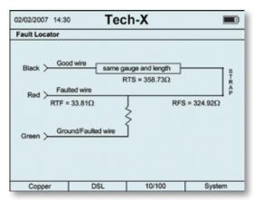
**Resistive Fault Locator**
