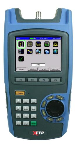
The TPNA-1000 measures a comprehensive set of digital signal parameters (Channel Power, MER, BER, Constellation Diagram), as well as analog signal performance characteristics (Single-Frequency Level, Scan, Tilt, HUM, C/N, Depth of Modulation), and Spectrum Analysis. In Level and Fast Spectrum Modes, the Peak-Hold function detects intermittent interference as a troublshooting aid useful in HFC network construction and maintenance.
