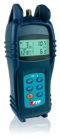
Single frequency mode displays the frequency and level of the audio carrier for an analog channel, or the center frequency and level of a digital channel. The TR-3 can be manually tuned to any frequency (46 MHz to 1 GHz) in steps of 50 kHz, 100 kHz, 1 MHz, 10 MHz, or 100 MHz.
