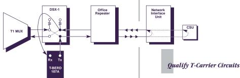
Utilize pre-programmed loop codes for intelligent repeaters to sectionalize span problems before dispatching maintenance personnel. Loop NIUs and CSUs from the central office with one test set. Perform automated pattern tests to quickly test the span and identify problems.
