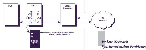
Timing problems are easily identified. Compare T1 circuit against a network reference clock to isolate timing slips.
