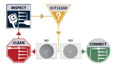
Contamination is the number one reason for troubleshooting optical networks. Proactive inspection and cleaning of fiber connectors can prevent poor signal performance, equipment damage, and network downtime.
